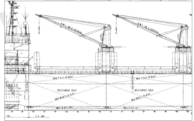
(Capacity plan section showing the layout of the cargo holds and ballast tanks)
