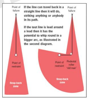
Ropes must never be left on warping drums after making fast. Snap back is common to all lines. Even long wires under tension can stretch enough to snap back with considerable energy. Synthetic ropes are more elastic therefore pose greater danger.
