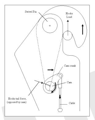
The diagram, showing the important features of resetting the mechanism, is complicated and makes it necessary to be able to clearly see the actual mechanism to understand its working.
