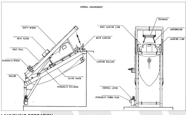
The boat is hoisted by the hydraulic winch and the boat to the specified position and the boat is stored by the hydraulic cylinders.
