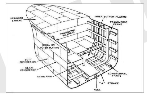
• **Keel**: the keel is a member, or series of members, running longitudinally that forms the structural base of a ship. The keel always corresponds to a ship's centreline. It is a major component in providing longitudinal strength and efficiently distributes local stresses when the ship is dry docked. There are two types of keels used to build ships of a certain size, the flat keel and the duct keel.
