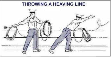
The heaving line should not be weighted by items such as shackles, bolts or nuts, or any other such objects; not attached directly to the heaving line and not inserted in the monkey's fist.
