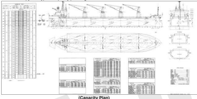
A copy of a typical capacity plan is given below:
