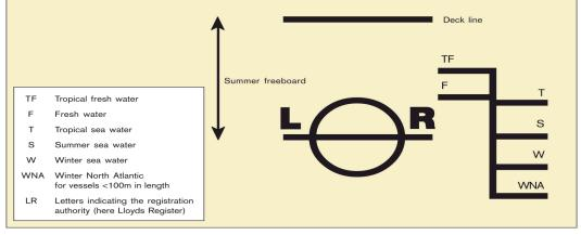
A ship assigned load line marks as shown above when in summer load line zone floating in seawater, of relative density 1.025 should not be submerged beyond the top of the 'S' line which is same as the top of the horizontal line running through the disc.
