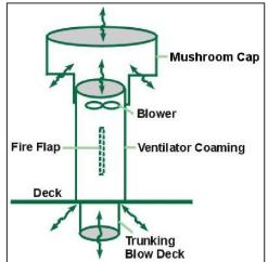
type of ventilation is in case of cargoes which give out flammable vapours. Any spark created by the motor may lead into an explosion or fire and hence the electrical motor and any electrical arrangement should be made intrinsically safe and flame proof. On modern ventilators a wire mesh is provided to act as a spark arrestor.
