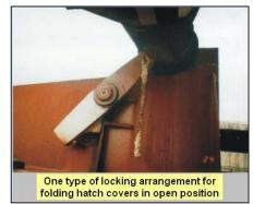
closing the hatch covers. The safety chain on single pull Macgregor type hatches does a similar job.
