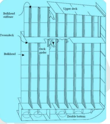
number and location of these bulkheads. But in general, there is a watertight bulkhead (collision bulkhead) at the bow that should be located between 0.05L and 0.075L (L = length between perpendiculars of a ship), a watertight bulkhead at the stern that should form a watertight aft compartment (after peak) that encloses the stern tube, and a watertight bulkhead at each end of the machinery space (where the aft bulkhead may be the after-peak bulkhead).
