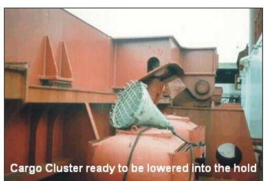
• When working in an area where the atmosphere is suspect, only "certified" and ' intrinsically safe" lamps should be used.
