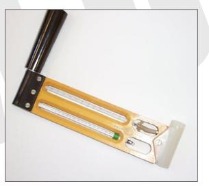
wick, cooling the wet-bulb thermometer. Then, the temperatures of both thermometers are read.
