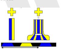
Figure 7: Emergency Wreck Marking Buoy
