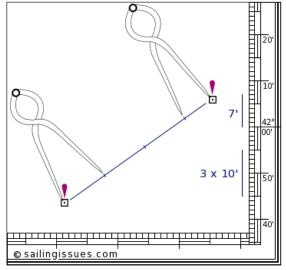
This device enables us to take the distance between that particular position and the closest grid line (latitude/ longitude). Then the dividers are placed on to the scale on the side with one end on the same grid line, and letting us measure the coordinate on the other end. This way we can get both latitude and longitude at the scale given on the edge of the chart.
