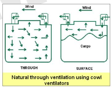
into the wind and the windward ventilator away from the wind, thereby achieving a greatest air flow rate which is required for through ventilation. Some cargoes like Rice bags are stowed in blocks to encourage through ventilation.
