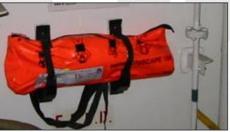
minutes, only used for escape from a compartment that has a hazardous atmosphere. They shall not be used for fighting fires or entering oxygen deficient voids or tanks. In these events, a self contained breathing apparatus, which is suitable for such applications, shall be used.
