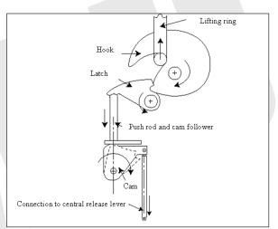
The diagram, showing the important features of resetting the mechanism, is complicated and makes it necessary to be able to clearly see the actual mechanism to understand its working.
