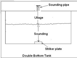
generally advisable to take ullage readings. Ullage is the vertical distance between the surface of the liquid and the top of the ullage plug or the top of the sounding pipe. The following diagram describes the relationship between sounding and ullage
