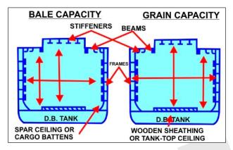
**22) Grain capacity**: This is the capacity of the space to load free flowing cargo like grain, iron ore, coal, and fertilizers in bulk, which will occupy any available space even in between frames spaces and can flow in to all corners of the hold. This capacity is the volume of free space available in a cargo compartment. It is the cubic capacity of the space where lengths, breadths and depths are taken right to the plating. An allowance is made for the volume occupied by frames and beams.
