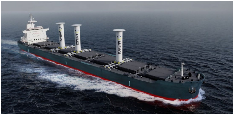
Figure 1: Illustration of Rotor Sails to be installed on Bulk Carrier in 3Q2023 ( Image courtesy of AMT )
