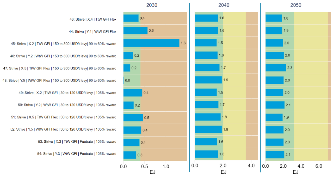
Figure D-40: Biofuel demand in blue bars for each scenario compared to the estimated supply of advanced biofuels available for shipping in 2030, 2040, and 2050, per scenario. The green to yellow boundary indicates the median estimated supply and the yellow to red boundary indicates the high estimated supply (Ricardo & DNV, 2023). Note that the x-axis scale changes between the years.
