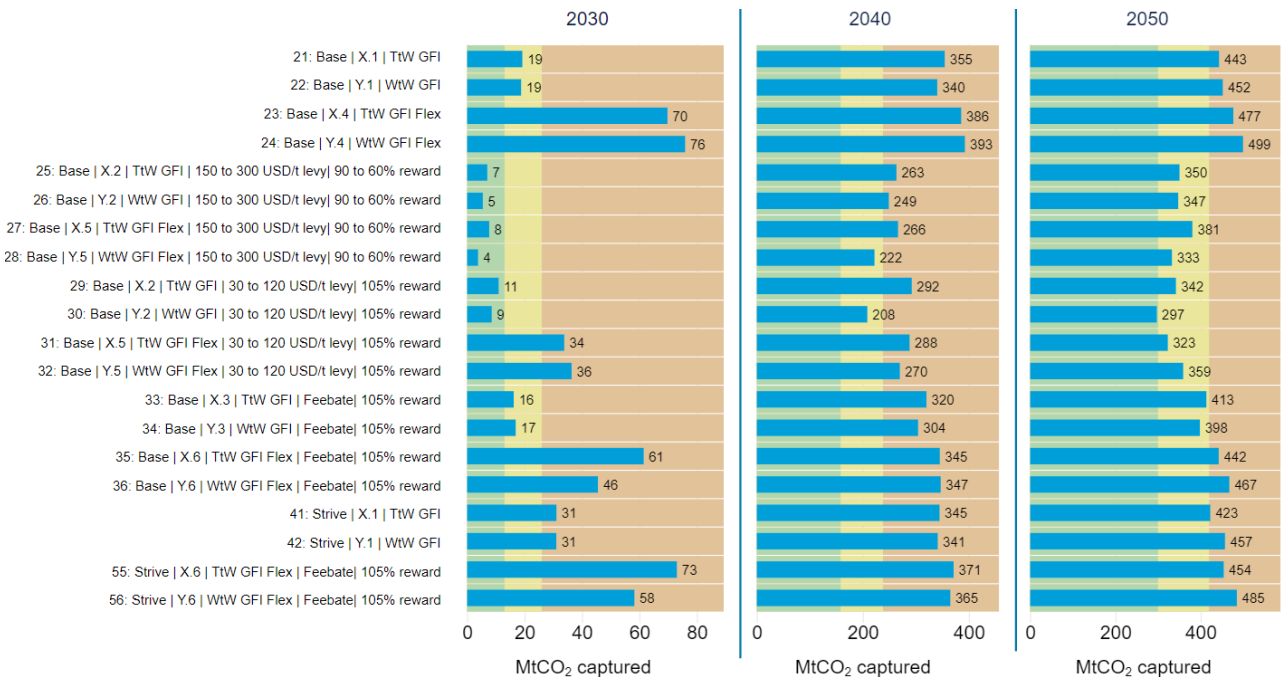
Figure D-28: Captured carbon storage demand in blue bars compared to estimated carbon storage capacity available for shipping in 2030, 2040, and 2050. The green to yellow boundary indicates the median estimated capacity available for shipping and the yellow to red boundary indicates the high estimated capacity available for shipping (Ricardo & DNV, 2023). Note that the x-axis scale changes between the years.
