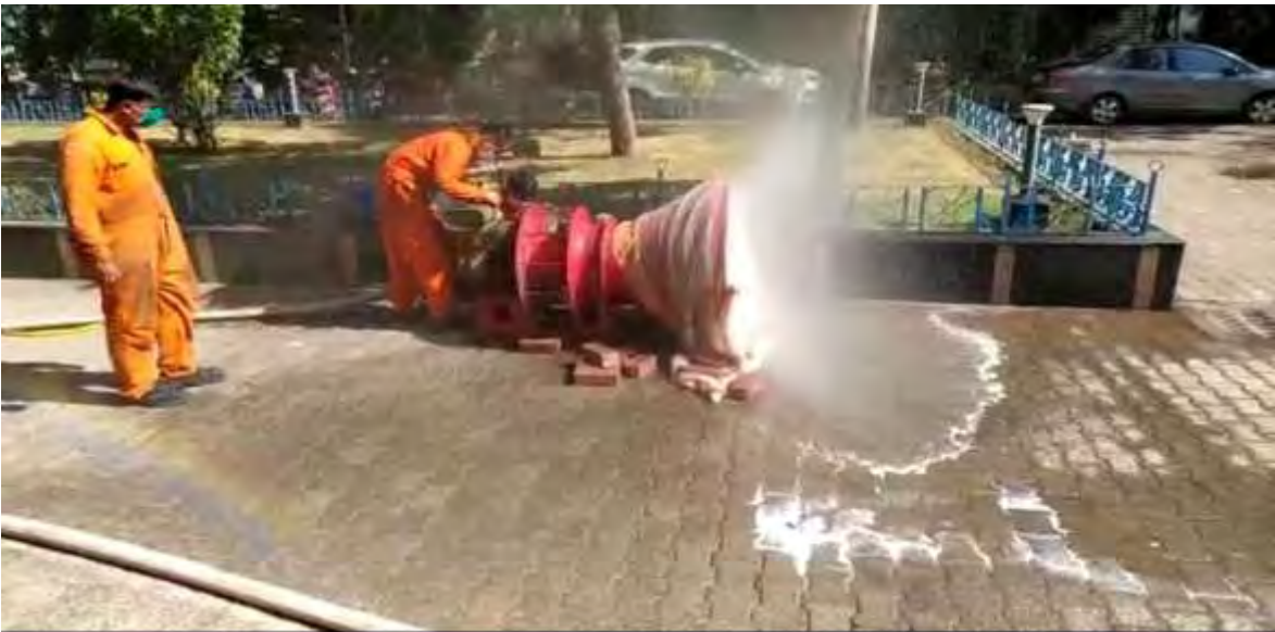
High Expansion engine driven foam generator in use
